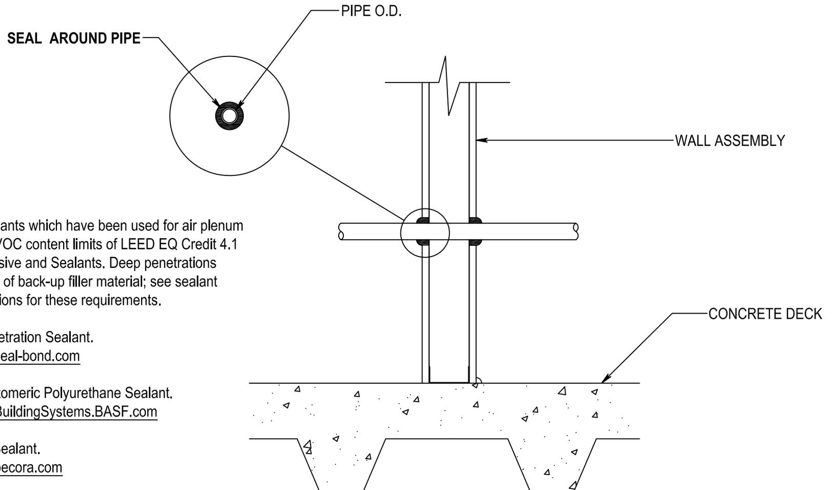
Following are Gun-grade sealants which have been used for air plenum sealing and comply with the VOC content limits of LEED EQ Credit 4.1 Low Emitting Materials: Adhesive and Sealants. Deep penetrations must be controlled by the use of back-up filler material; see sealant manufacturer's recommendations for these requirements.
